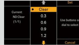
Quick access for setting FPS, EI, Shutter, ND, Look and WB by six buttons at Sub Display top and bottom
