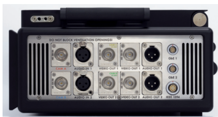
PSU-3 input/output panel to connect four cameras, two sound signals and up to four monitors.
