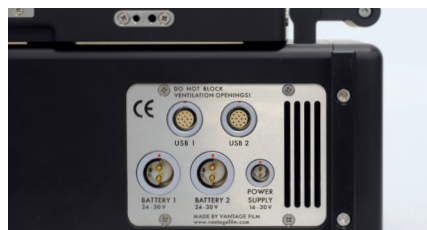
The PSU-3 can be powered by camera batteries (24-30V) or through a compact power unit.
