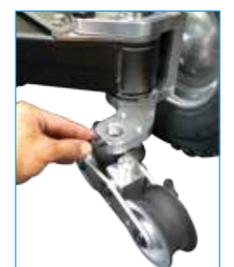
quick lock for easy wheel change
