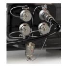
When connecting or disconnecting the cables **grip the connector bodies**. Do **not** pull on the cables, as this will damage the connector assembly
