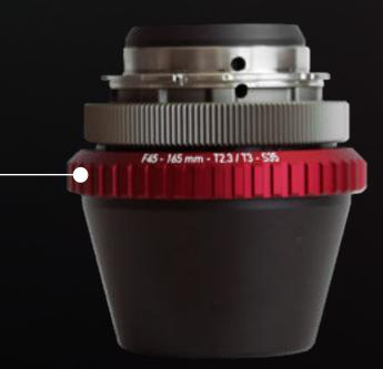
1. EZ Change of the image format coverage by unlocking the red nut, going from FF to S35. Swap the rear and relock.
